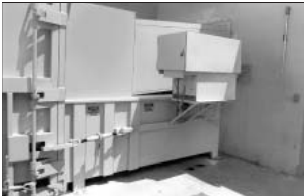
Rear Load Security Chute & Side Mounted Power Unit
