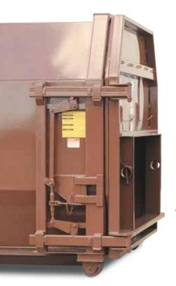
This Wet Pack System includes a CP-2102 compactor (raised 4" and equipped with a pinning/boost override system and a pinning tunnel mounted on the ram face). The system also includes a compaction container with an optional adjustable sealed door and a raised compaction opening, pinning tunnel and binder pockets to match the compactor.
